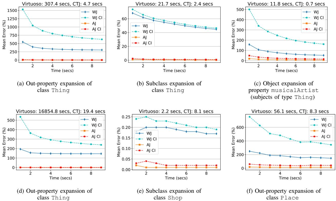
Fig. 8: The MAE per second of the estimators (WJ and AJ) and 0.95 confidence intervals (WJ CI and AJ CI), as well as exact runtimes (Virtuoso and CTJ) for a selection of exploration queries: from DBpedia (top) and from LinkedGeoData (bottom)
