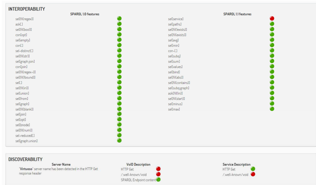
Fig. 5. Screen capture of the detailed view for the DBpedia endpoint ( http://dbpedia.org/sparql ) showing the results of interoperability (individual queries passed or failed) and discoverability tests (locations of VoID and SD descriptions) in the most recent run.
